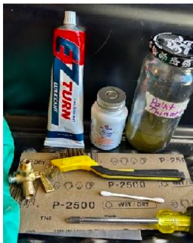
Above Right: What's needed to clean and reinstall the valve. Photos provided by Don Neidigk, September, 2024.
